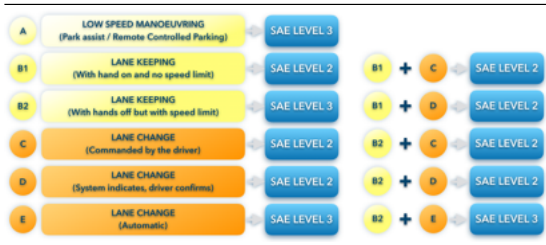
Fig: 1.7: Correspondence of UNECE autonomous function categories with SAE levels of automation
