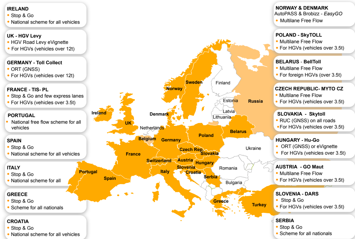
Fig. 1.5: Electronic toll collection schemes for trucks in Europe
