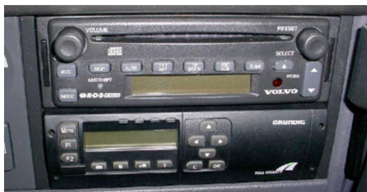
Figure 126: A Grundig OBU, installed on a truck for the German Toll-Collect system
